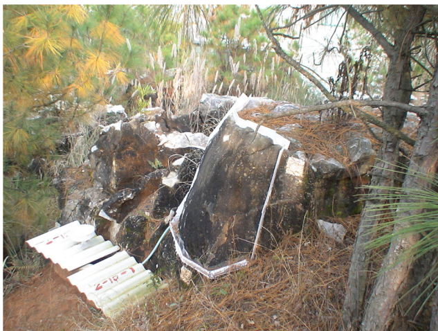
Fig 1 Runoff water collection systems, polyvinyl chloride (PVC) strips were inserted into grooves and sealed by silicon sealant to enclosed rock surface with an area of approximately 1 \text{ m}^2 . An L-shaped aluminum foil strip was attached to the bottom PVC strip surfaces to form a trough with a gradient of 20\text{--}45^{\circ} , leading by means of polyethylene tubing to a 15-L barrel set in a hole in the ground
